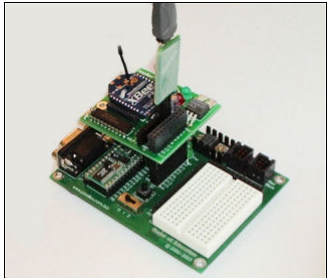
XBee-PRO mounted on AppBee-MOD using USB2SER for PC communications.
